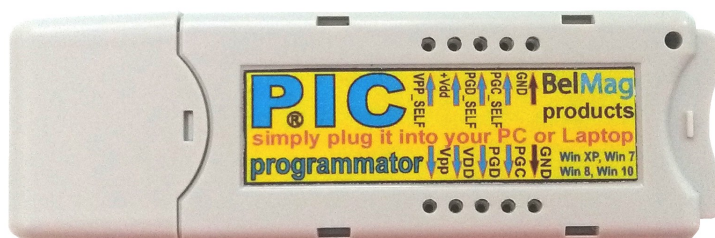
Slika 1. USB ICSP PIC programator.
