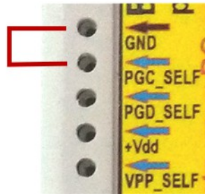
Figure 7. Firmware loading/upgrading mode configuration.
